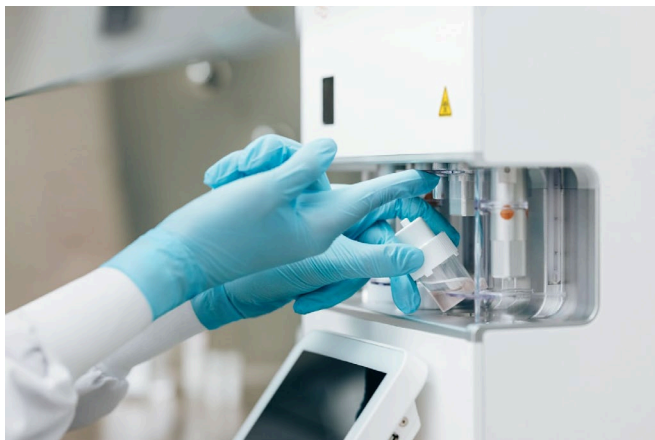
Figure 35. Loading the STEMprep™ Sample Tube
