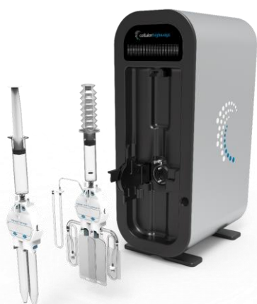
Figure 1: The Highway1 cell sorter and sterile cartridges.
